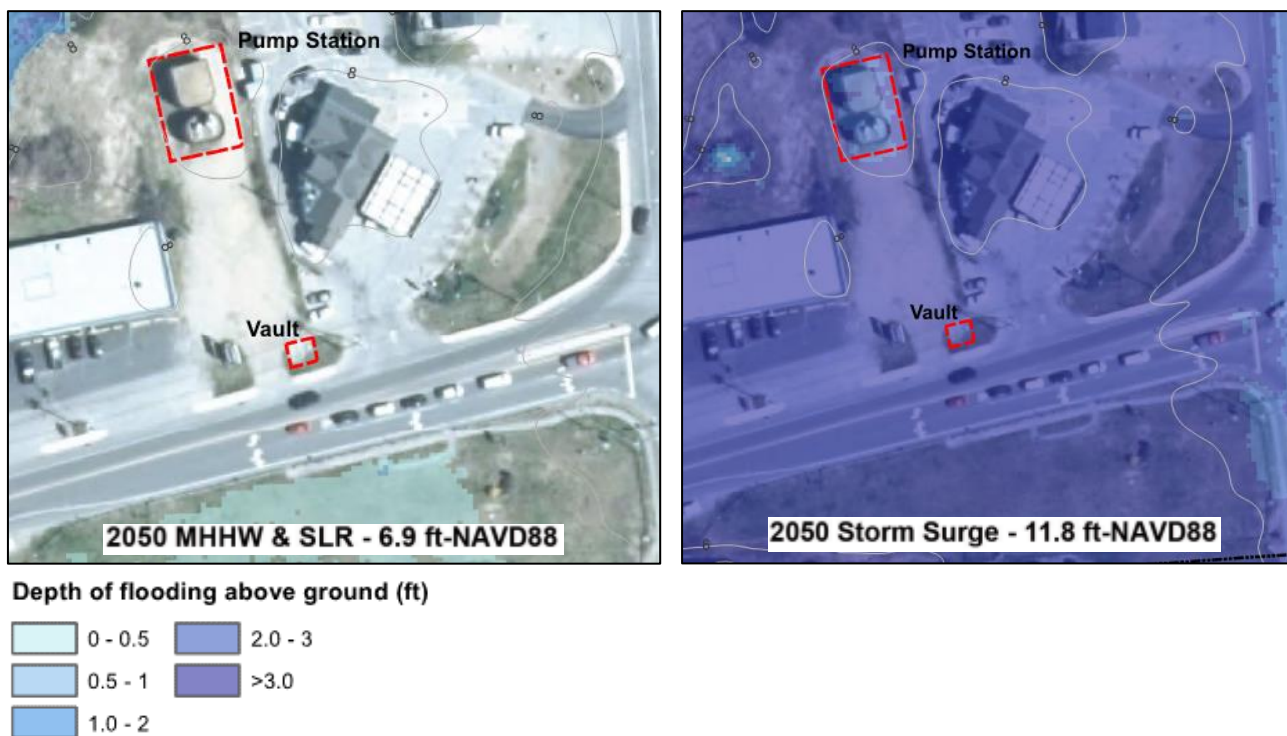
Figure 3-3: Storm surge Conditions at the Pump Station in 2050
